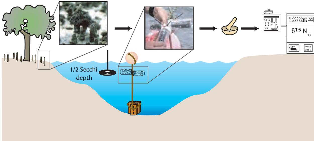
Collect macroalgae (or other indicator organisms such as oysters or submerged aquatic vegetation) from a site distant from nutrient sources, incubate *in situ*, then dry, grind, and analyze on a stable isotope mass spectrometer for determination of  $\delta^{15}\text{N}$ .
