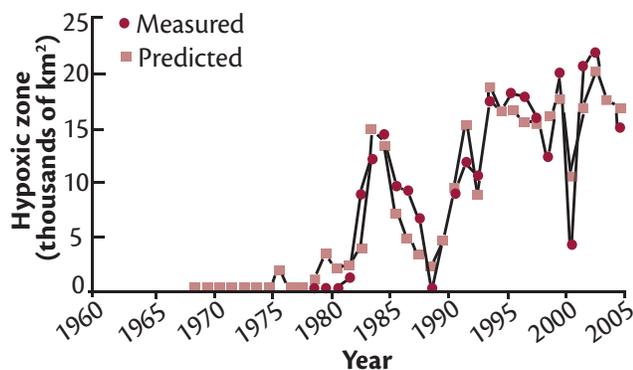
\*The results of a model predicting the size of the hypoxic zone from 1968–2004. The equation is:  $y(\text{km}^2) = -1337953.4 + 672.1589(\text{Year} + 0.0998)$  (May flux as nitrate + nitrite), (Turner et al. 2006).
