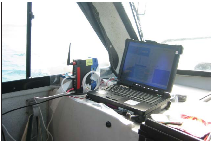
Figure 3.5. Tracking equipment and computer set up for AUV deployment. Photo: NOAA/NCCOS/CCMA Biogeography Branch.
