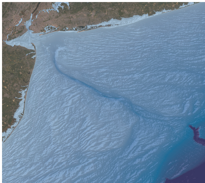
Image 2.1. An example of a bathymetric surface in the New York Bight, showing the change in depth with distance from shore and the complexity of the seafloor across the shelf. The Hudson Shelf Valley is prominently visible in the center of the model as the area of darker blue extending from New York harbor (top left) towards the shelf edge (bottom right). Coastal managers and engineers use bathymetric surfaces to assess shipping lanes, identify fish habitats, lay undersea cables and find sand and gravel resources. The bathymetric surface shown here is the NOAA Coastal Relief Model (CRM), draped over a derived hillshade layer to highlight bathymetric variation. Terrestrial imagery is the ArcGIS Online World User Imagery layer (ESRI Online).
