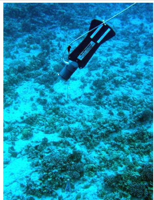
Figure 8. Video Drop Camera used to observe and record benthic characterization data.
