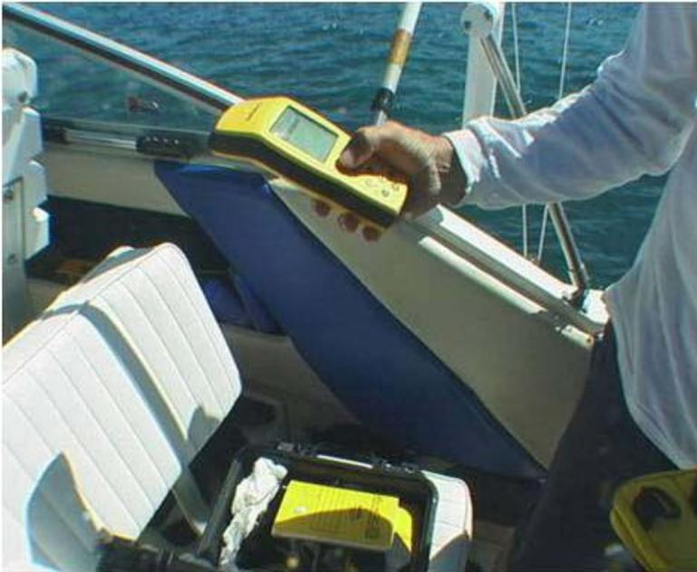
Figure 6. Field data collection on a Trimble GPS data logger.
