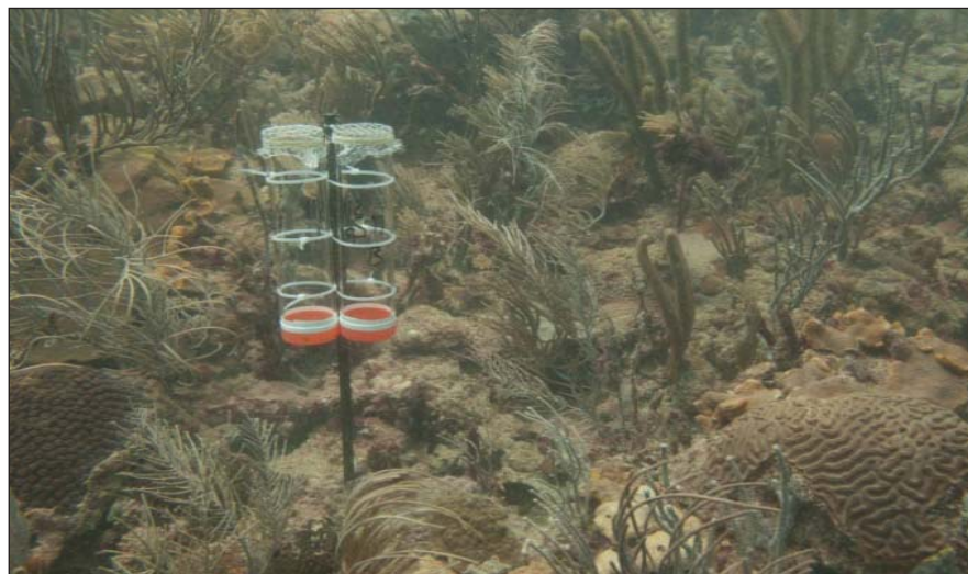
Figure 4.2. Simple tube traps used to collect suspended sediments. Sediment traps were clear plastic tubes 30-cm high with an internal diameter of 6.4 cm. Tops of the traps were covered with a 1\ \text{cm}^2 nylon mesh to prevent entry of small fish and invertebrates. Traps were secured with plastic cable ties to steel rods that were driven into the hard reef surface. Traps were situated so that the tops of the traps were ~60 cm above the surrounding seafloor.
