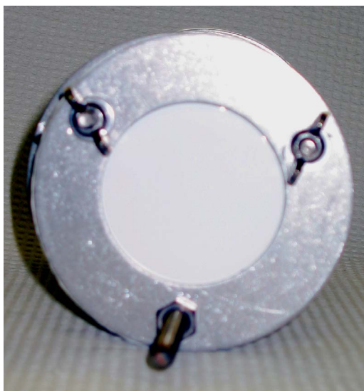
Figure 6.1. Example of a POCIS disk. Image courtesy of the USGS.
