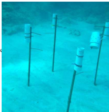
Sediment traps deployed in the STEER. Larger cylinder is a passive water chemistry sampler used in another part of the project (see Chapter 6).
