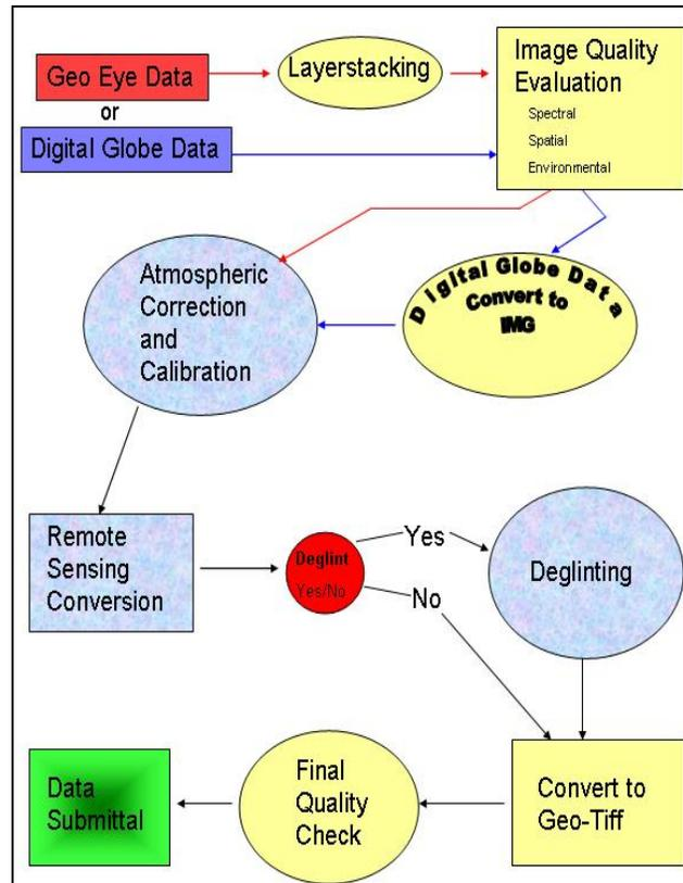
Figure 1. Image processing flowchart for IKONOS and Quickbird data. Only the image processing portion of data flow is shown. Additional steps such as creation of mosaics and metadata are described in the upcoming text.
