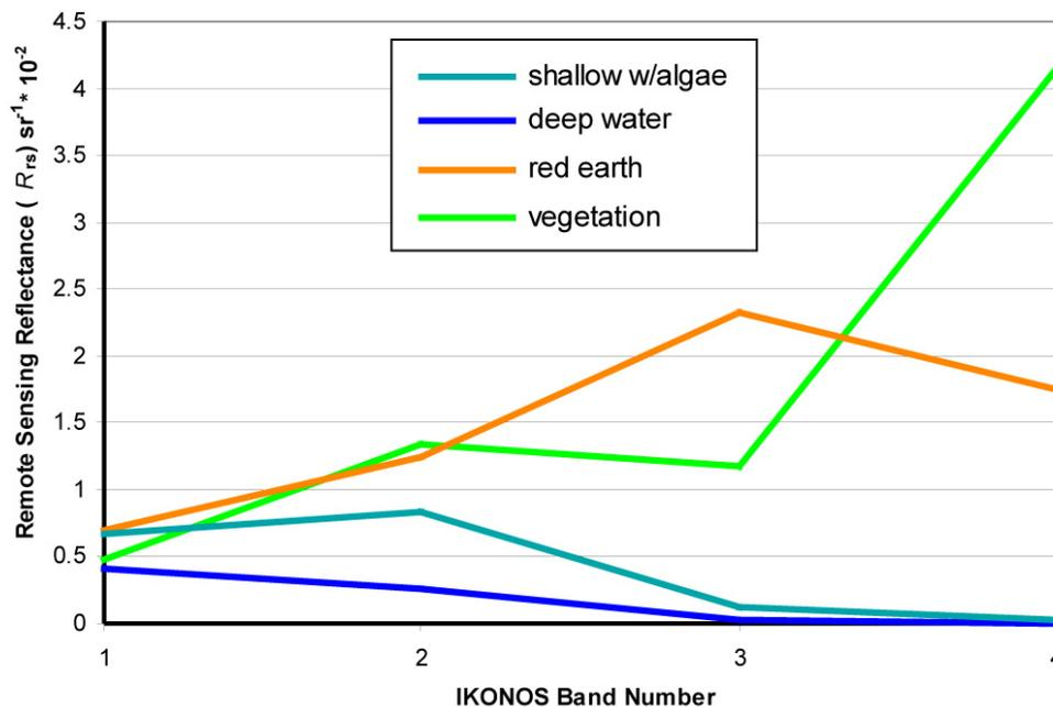
Figure 2. Example remote sensing reflectance spectra of seafloor and ground cover.
