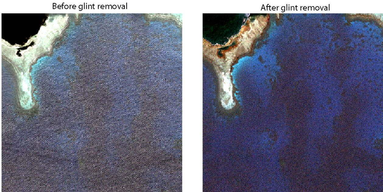
Figure 3. An example of deglinted output. Before the deglinting algorithm was run, glint was a major problem when trying to classify bottom features, such as small coral outcroppings in the deeper water outside the reef shelf. Also visible were tracks made by the wake of a passing boat in the bottom left corner. After deglinting, the image is much clearer and easier to use in bottom classification. The boat wake has also been removed.
